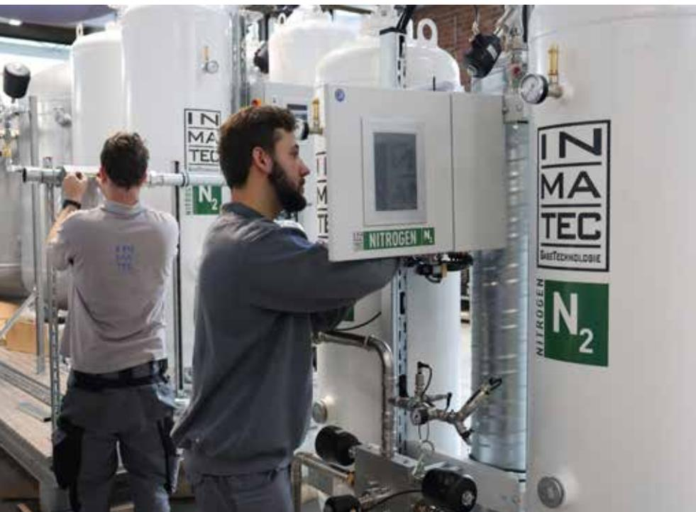
The IMT PNC from Inmateg generates nitrogen with a food compliant purity of 99.5% directly on-site from the ambient air and makes beverage manufacturers independent from carbon dioxide and carbonic acid supply bottlenecks.
