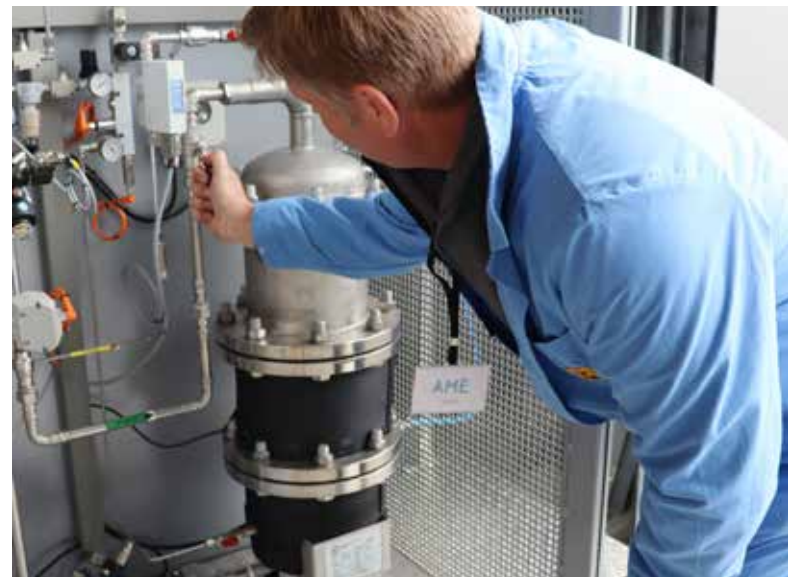
The nitrogen obtained is enriched with small amounts of hydrogen in the NKat hydrogen catalyst and thus brought to a purity of 99.999% in an energy-saving manner.
